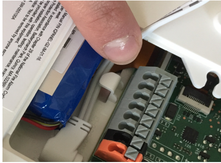
Route the wire behind the retainer clip
