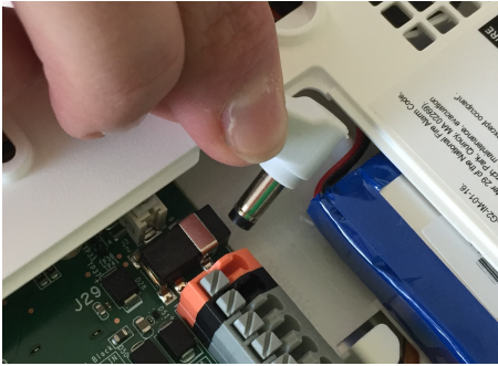
Plug in the power connector
